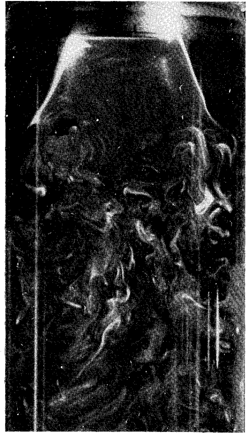
Fig. 3 Flow visualization for combined wake and recirculation zones: \phi = 70 deg, \beta = 11.8 , Re = 1352 .
